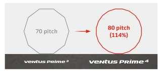
By increasing the total number of pitches, the impact on the road surface is minimised providing a more comfortable ride.
