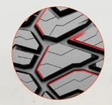
Stepped chamfer on tread blocks for smoother on-road running and stable braking under force.
