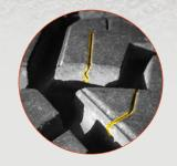
3D tread sipes allow the tread blocks to work independently to allow extra biting edges when the vehicle is off road, but lock together under force for more stable braking.
