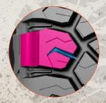
Dual-part shoulder tread block with extra deep clearance groove for multiple extra gripping edges.
