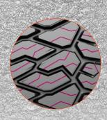
Multi-angled tread sipes provide extra biting edges and allow the tyre to mould to the terrain in rough conditions.
