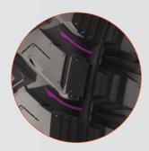
Razor mud and stone ejectors on shoulder groove for extra grip and reduced tyre damage.
